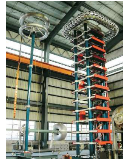
345kV ultra-high voltage cable impulse withstands voltage testing
