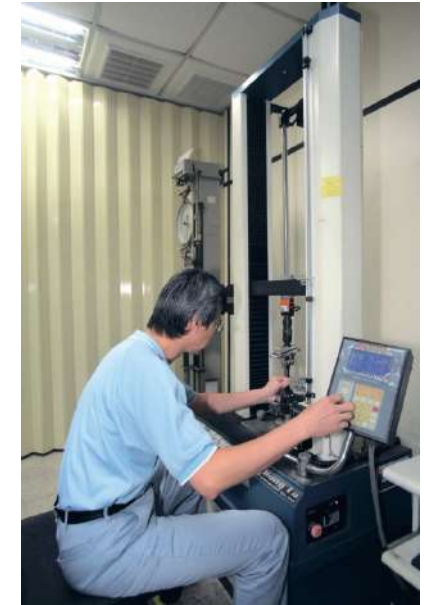
Wire and cable material tensile and elongation testing
