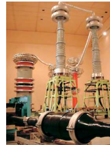
61kV withstand voltage testing
